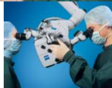
(above right) Rotation of both binoculars in cross-table procedures ensures proper ergonomic positioning, even when the OPMI is positioned at an angle.
