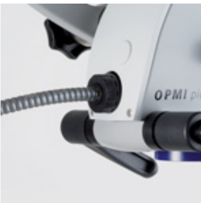
Orange filter. Prevents premature curing of composite materials.
